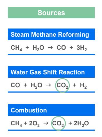
1 kg of  $H_2$  production typically emits 8-12 kg  $CO_2$  (grey hydrogen)
